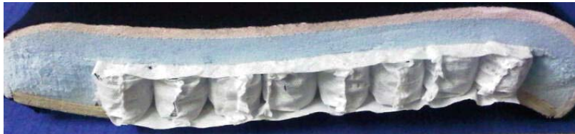
Cross Section of Posturepaedia Seat showing Pocket Springs and top layer of Memory Foam
